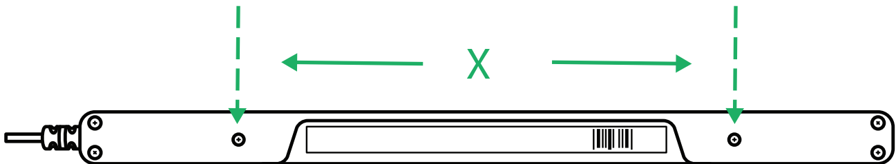
Figure 4.1 C-C Distance Between the M3 Screws
